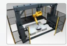
3D and 2D application, optional gantry can be equipped with a 2-D cutting platform, can achieve 3-D cutting and plate cutting functions on the same equipment.
